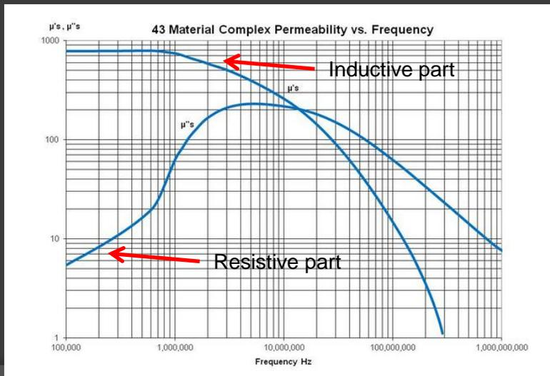
Permeability is actually complex - it has an inductive component ( $\mu'$ ) and a resistive (lossy) component ( $\mu''$ )
