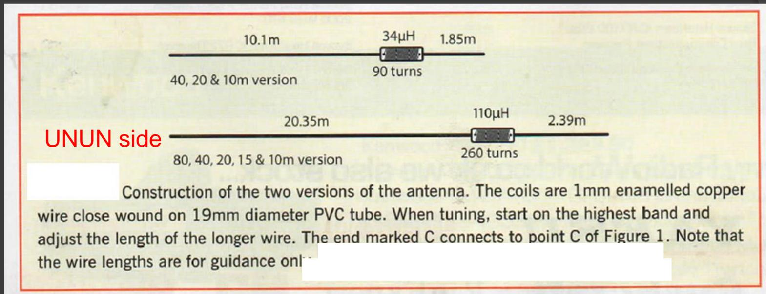
34uH coil: 90T, 110uH coil: 260 turns, 1mm (AWG #18) wire on 19m PVC tube. Adjust the long wire first for the high end bands. Then adjust the short wire for the lowest band.
