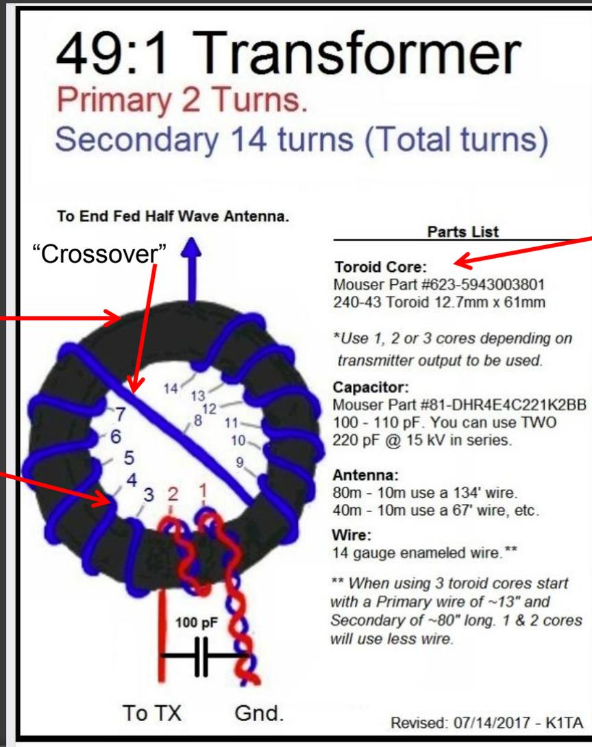
I recommend 2 type 43 material for less than ~250 watts for lower cost, Fair Rite P/N 5943003801
