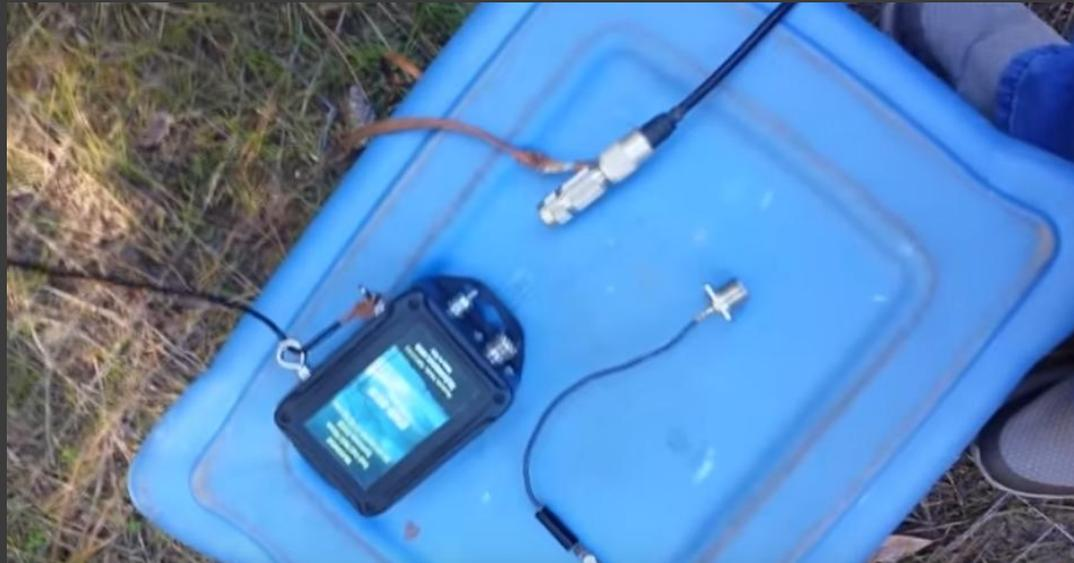
Disconnect UNUN from coax feed. Connect jumper between coax feed and antenna, leaving UNUN “float”. The EFHW becomes a quarter wave antenna on 160 meters. Needs a good ground system to work properly.
